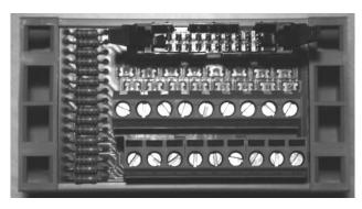
XEL is the corresponding wiring interface for logic inputs on the XIO board. The board includes filtering and protection to prevent damage from external AC sources. Status indicators (LEDs) provide an easy way to see the state of each input. A flat ribbon style cable connection is used for simple installation.
