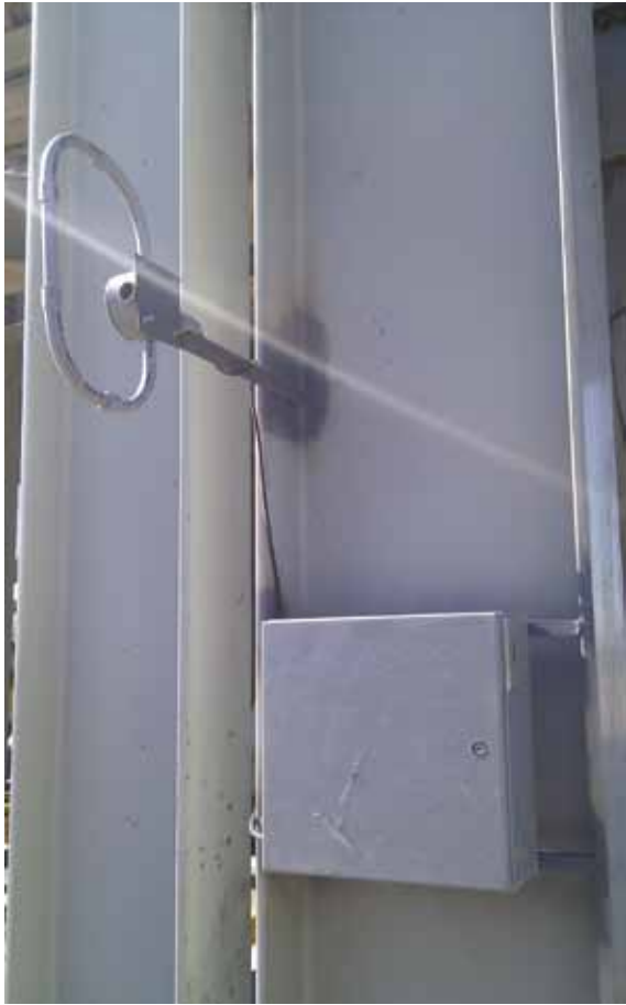
ABOVE: This is the marker loop antenna on the side of one of the silo legs at the Wichita, Kan., plant location. BELOW: This arrow points to a PaveTag tag correctly installed on a haul truck.
