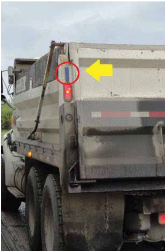
ABOVE: This is the marker loop antenna on the side of one of the silo legs at the Wichita, Kan., plant location. BELOW: This arrow points to a PaveTag tag correctly installed on a haul truck.
