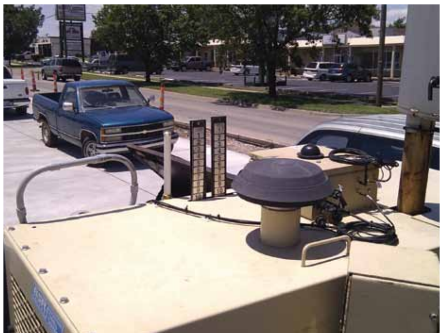
The top of this Lafarge paver includes a marker loop antenna and long range antenna on a jobsite in Wichita, Kan
