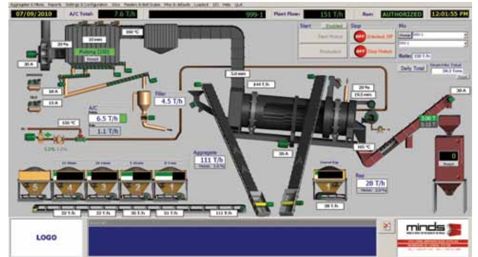
The DrumTronic system allows plant operators the option of one to four screens that display bar graphs, plant configurations, charts, and more to give a quick and easy snapshot of the plant's status.
