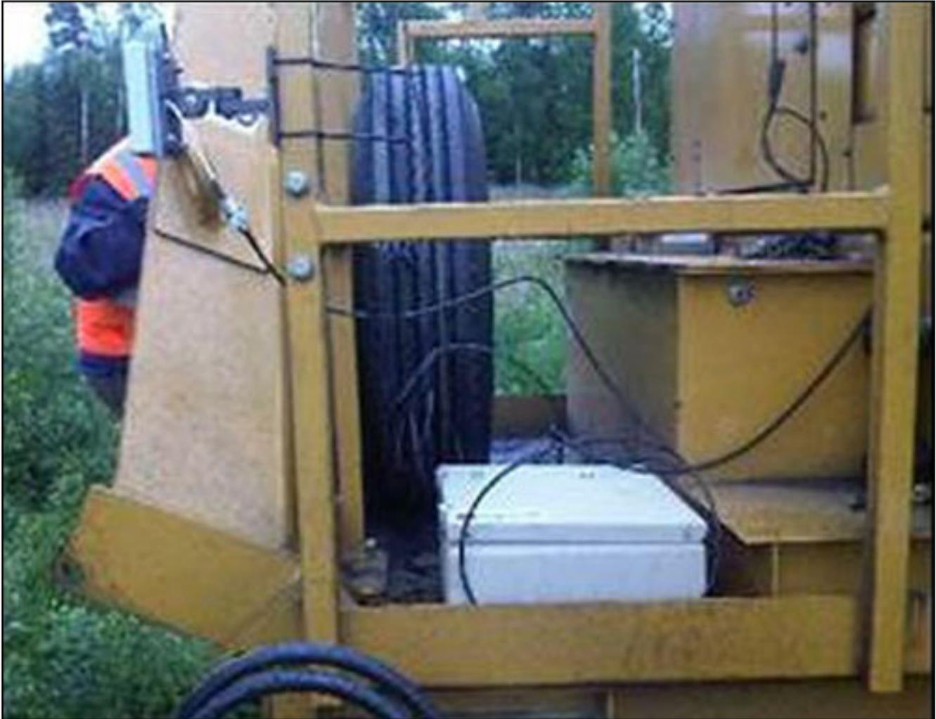
*An Identec RFID reader and antenna were mounted to the rear of the paver.*
