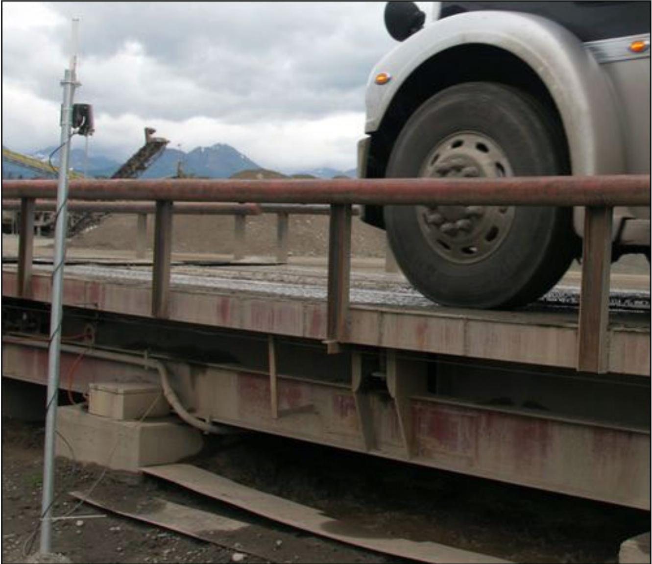
*An Identec reader mounted on a pole near the entrance of the scale captured the RFID tag transmissions of a loaded truck.*
